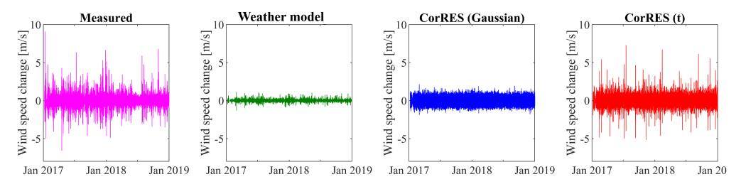
10 min wind speed ramps in measured data (magenta) and in different stages of the CorRES simulation procedure: interpolated from hourly weather data (green) to the final result with stochastic simulation included (red)
