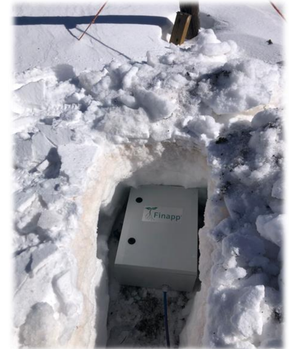
"On-ground" probe for Local SWE measurements
