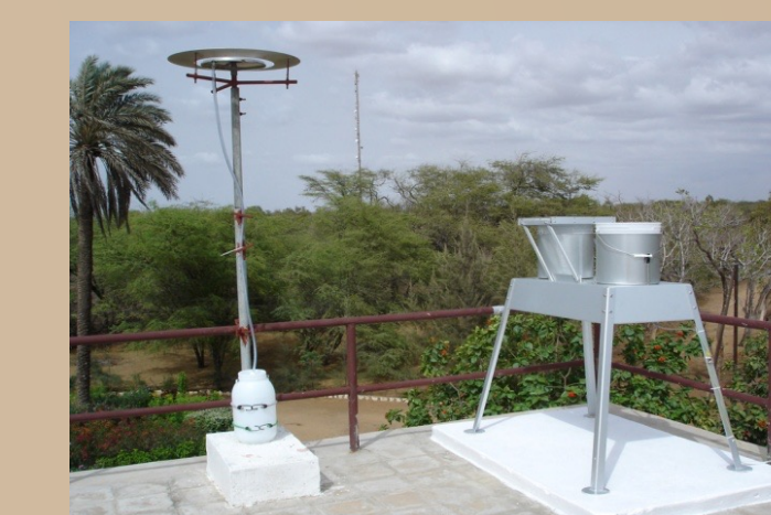
Total (left) and wet (right) deposition collectors deployed in the INDAAF network.
