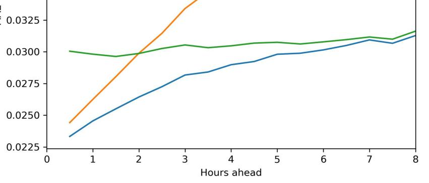
MAE per forecast horizon for PVNet-2 with various inputs
